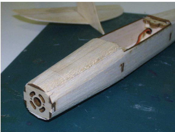
Figure 4.14: Front of fuselage shaved to shape
