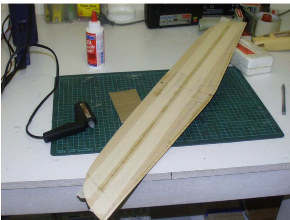
Figure 3.6: Masking tape applied for hotglue tips
