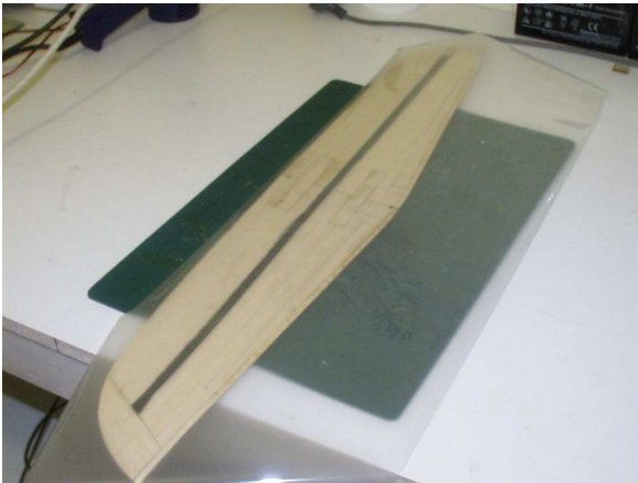
Figure 3.8: Wing being covered
