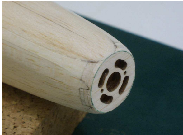
Figure 4.17: Nose sanded to smooth profile
