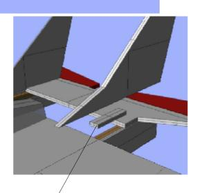
fill the little gap with a piece of depron in order to obtain a level surface and then hot glue the fins in place
