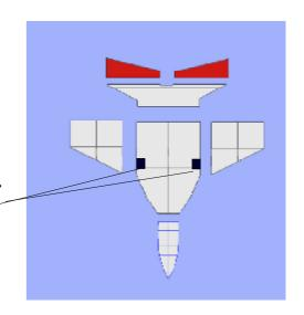
cut out slots for the servos and hot glue nacelles to body (balsa) and tail.
