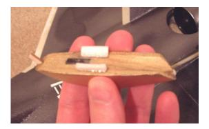
Add tabs from scrap material to attach the canopy to the forward fuselage.
