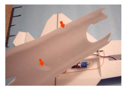
Test fit the panel and make adjustments as needed. Check the inside of the panel for marks that indicate interference with installed components and sand small clearance pockets if required. It's important that this panel is installed without a lot of tension or the wing and chine area will warp.
