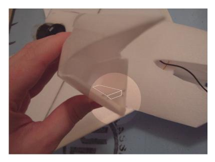
**30** – Glue the forward fuselage in place. Sight down the model and aim the rearward point at the center of the fan.
