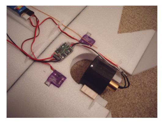
**TAKE YOUR TIME HERE!** I have wrecked a lot of models because the thrust line of the fan was set incorrectly. Use a drafting triangle or similar tool to get the fan case perfectly aligned with the centerline of the model.
