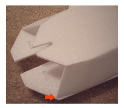
**5** – Bevel the lower forward edge of each elevon and hinge them to the wing with Blenderm tape on the upper and lower surfaces.
