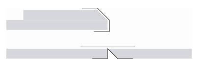
6 – Glue fuselage formers in place on the upper surface of the wing.
