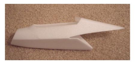
**23** – Bevel the edges of the forward fuselage assembly and upper skin as needed for a gap free fit and glue in place.
