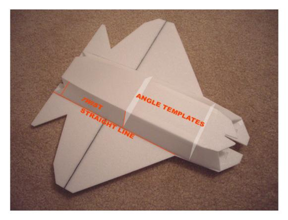
**4** – Bevel the top edges of the lower fuselage cover so that it fits flush with the underside of the wing. Eliminate any twisting that will warp the wing. Glue the lower fuselage cover in place as shown then make the lower fuselage fan cutout. Note the pictured misalignment of the chine and intake edge - this is a scale detail.
